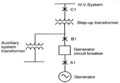
Fig.3.4 Single-line diagram of unit generator system
